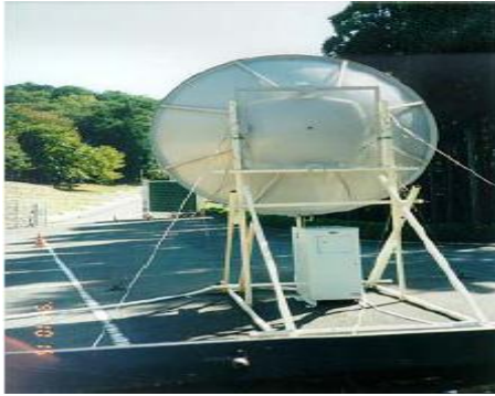
Fig. 4. Ground-to-Ground MPT Experiment in Japan in 1994-95
