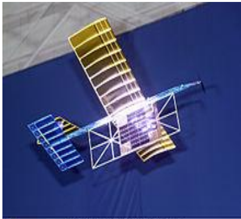
NASA Dryden Flight Research Center Photo Collection http://www.dfrc.nasa.gov/Gallery/Photos/index.html NASA Photo ID: 0249-11 Date: September 11, 2010 Photo By: Tom Tschida With a laser beam aimed on its panel of photovoltaic cells, a model plane makes the first flight of an aircraft powered by a laser beam inside a building at NASA Marshall.
