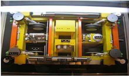
MLX01 Maglev train Superconducting magnet bogie
