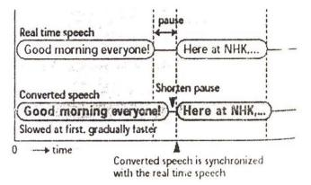
Speech signal is a complex signal consists of many frequencies Pitch is the perception of frequency .If the frequency of speech is affected by expansion the pitch will also varies. Care should be taken that naturalness of speech is maintained. The ASRC (Adaptive Speech Rate Control Algorithm) is used to achieve this .The technique used for expansion and contraction is insertion and deletion of pitch period and to maintain perceptual naturalness.
