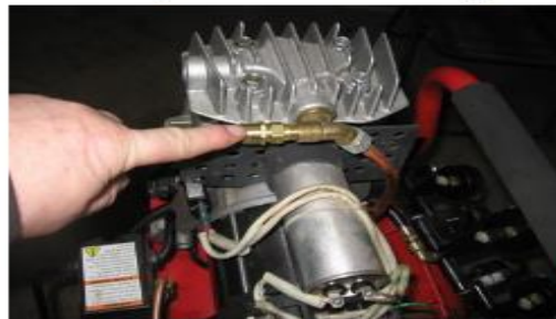
Safety Valve for Air Compressor
